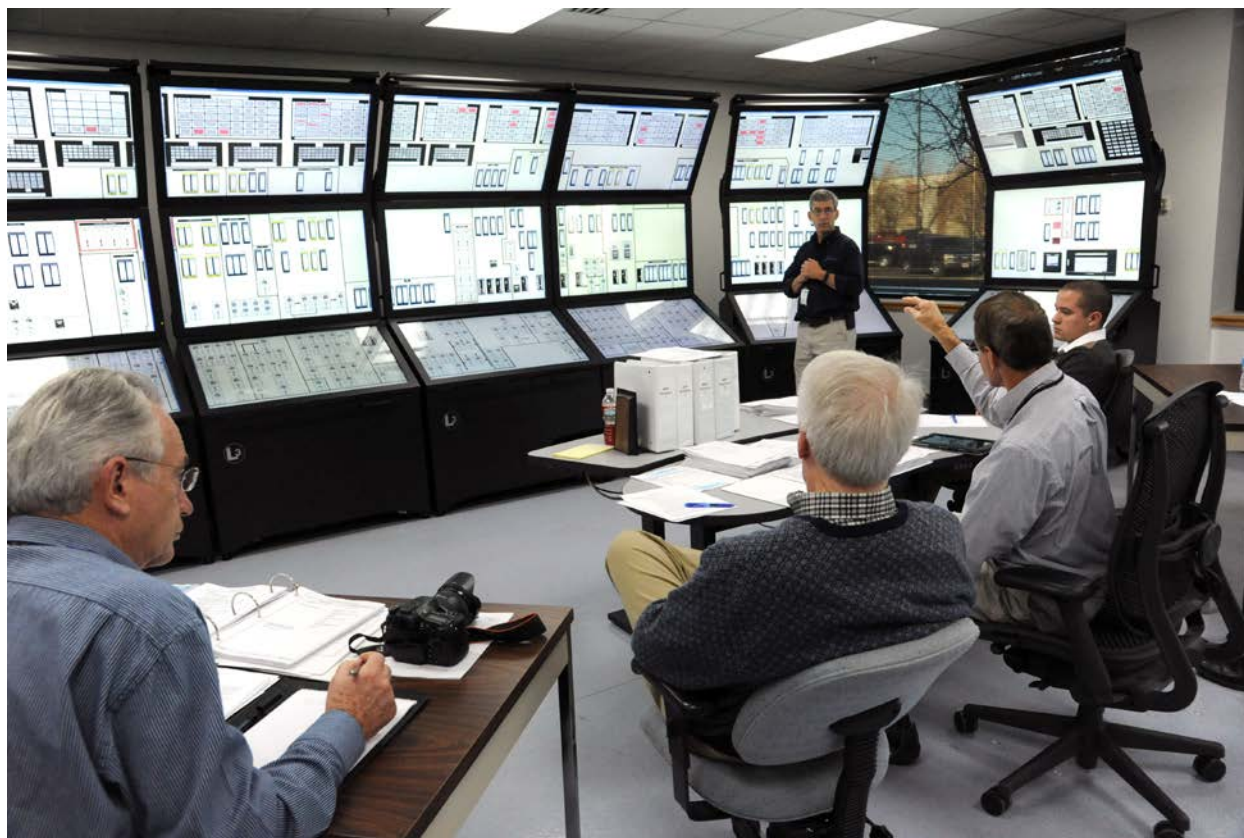
Figure 23. An operator workshop with a nuclear utility being conducted in the Human Systems Simulation Laboratory using the bench-board-style touch panel control bays.
