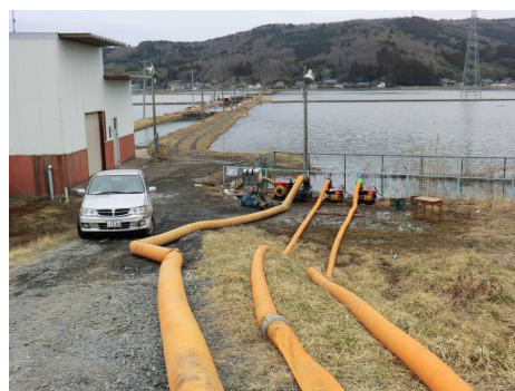
Disaster emergency pumps used to drain farmlands. (Ishinomaki, Miyagi Prefecture)
