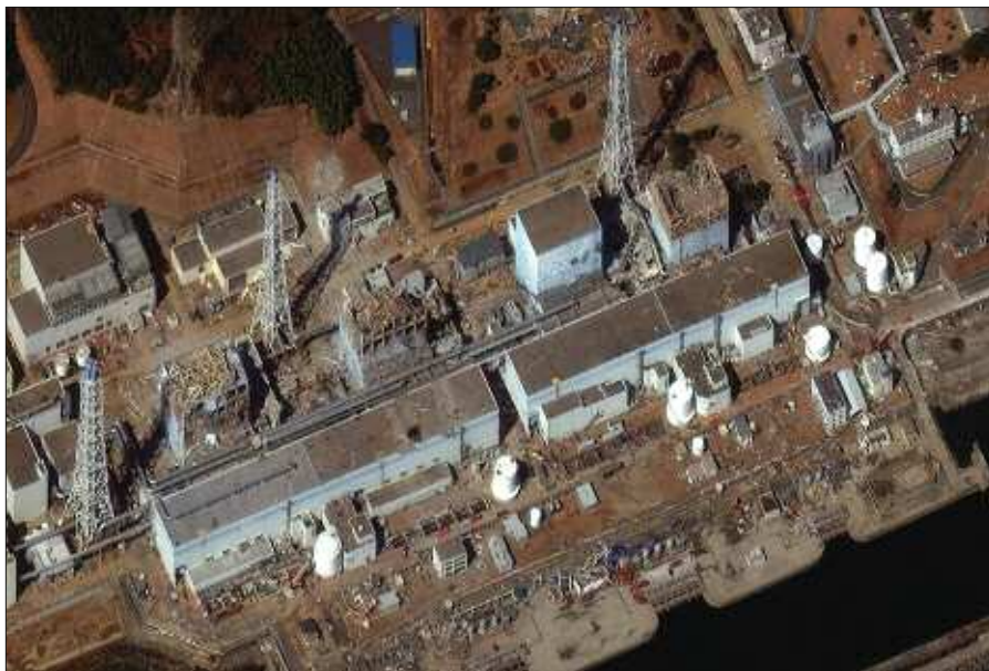
This satellite image, released by DigitalGlobe on March 18, shows the substantial damage to the external structures of the reactor buildings of (from left) Units 4, 3, 2, and 1 of the Fukushima Daiichi plant. The hydrogen explosions that caused the damage occurred outside of the reactor containments. (Photo: Reuters/DigitalGlobe/Handout)
